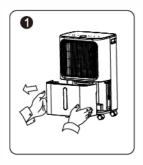
Hold the grooves on the left and right sides of the water tank with both handsat the same time, gently pull out the water tank. Please pay attention to keeping the water tank stable to avoid spillage.
