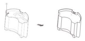
4. Clean the water tank and fully dry it. Then catch the cover and the handle to the water tank and reinstall the water tank.
