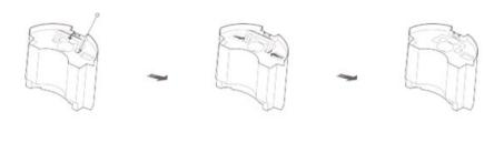
3. Remove the cover of the water tank from the spout on the top right corner of the water tank.
