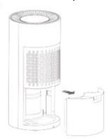
2. Remove the air inlet grille, and then remove the inner air filter.
